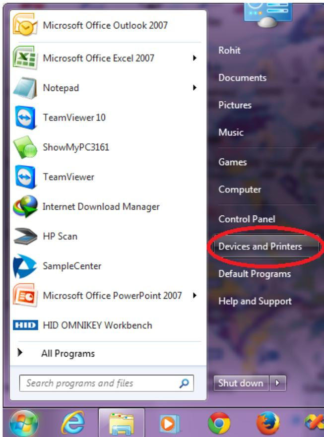
**STEP 2:** Find the active instance of “DTC1000 / DTC1250e Card Printer” → Right Click → Click on “Printing Preferences”.
